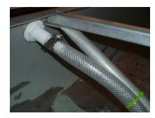
Finally, after the water is drawn through the strum box by the foot pump, it is ejected through the hull of the canoe as shown in this photo. There is nothing like waiting until race day to test some fairly important operational gear.
