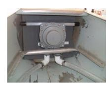
The photo on the right here is the part of the bilge system that intakes the water. It is the strum box. Trying to draw water on a virtually flat bottom boat is a feat in itself. We placed this box on the starboard side of the boat, so that when we lean that direction, the water will pool in that area. At least in theory.
