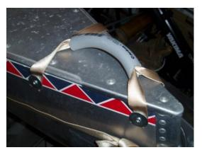
We spent this past week acquiring the remaining gear that we will need as well as making the final modifications to the boat. We moved the portage handles from their position hanging off the bow and stern to a sturdy mount on top of the bulk heads to eliminate drag
